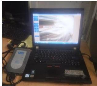
Gambar 5. Alat Toyota GTS (*Global Tech Stream*)
