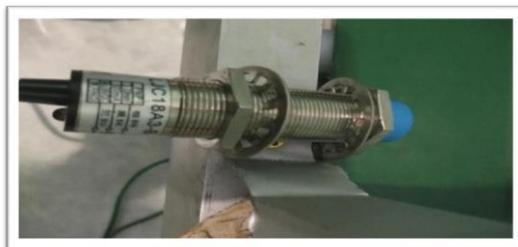
Gambar 8 Sensor Kapasitif Proximiti
