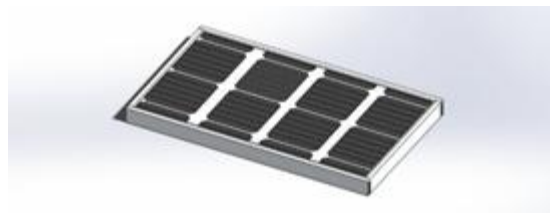
Gambar 2. 3D Geometri Panel Surya Kapasitas 50 Wp Tipe Monocrystalline.
