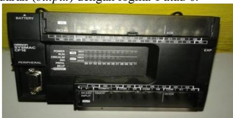
Gambar 3-2. PLC Omron Sysmac CP1E-N30SDT-D
