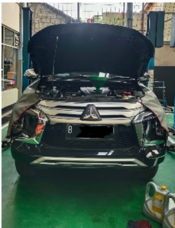
Gambar 2. Pemasangan Fender Cover
