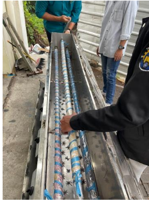
Gambar 4. Finishing Mesin Pengukus Kain Ecoprint
