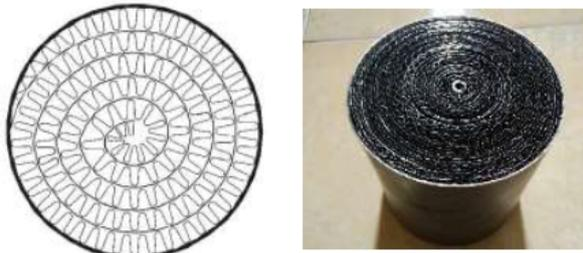
Gambar 6. *Chrome-coated copper* (Cu+Cr) *catalytic converter*. Diadaptasi dari (Warju et al., 2018)
