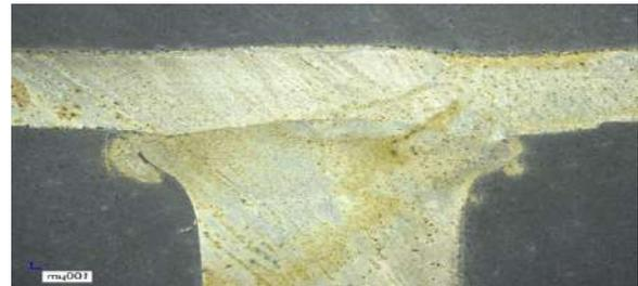
**Gambar 12** hasil *visual crack welding* keenam
