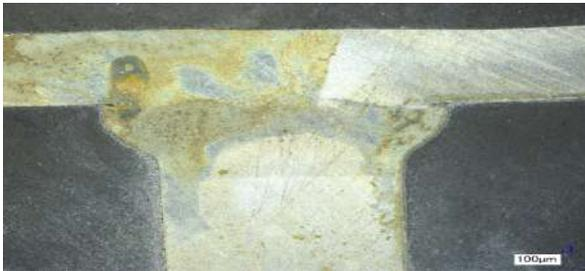
**Gambar 5** Hasil *Visual crack Welding* Pertama
