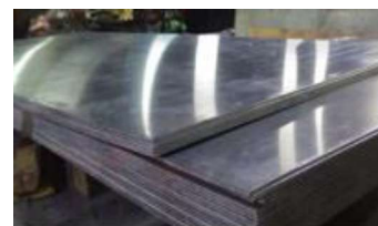
Gambar 1. Aluminium clad 2024 T0 0.071 inch
