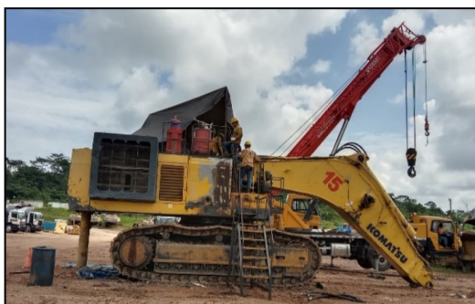
Gambar 1. Persiapan proses pelepasan recoil spring
