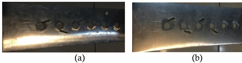
Gambar 4. Delta winglet vortex generators (a) staggered satu pasang, (b) staggered dua pasang
