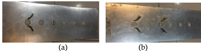
Gambar 5. Concave delta winglet vortex generators (a) in-line satu pasang, (b) in-line dua pasang
