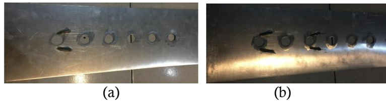
Gambar 3. Delta winglet vortex generators (a) in-line satu pasang, (b) in-line dua pasang
