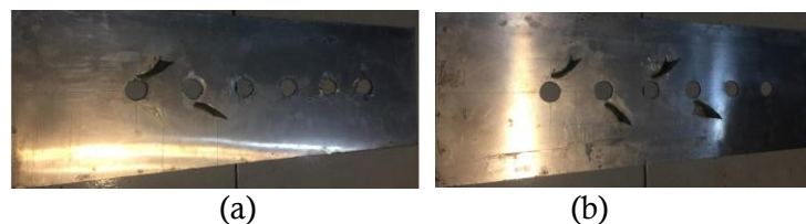
Gambar 6. Concave delta winglet vortex generators (a) staggered satu pasang, (b) staggered dua pasang
